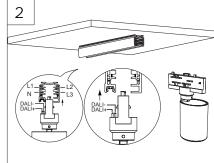
Track layout should be refer to the track installation manual.Turn "L" and "N" knob to perpendicular position to adapter before installing the fixture.
